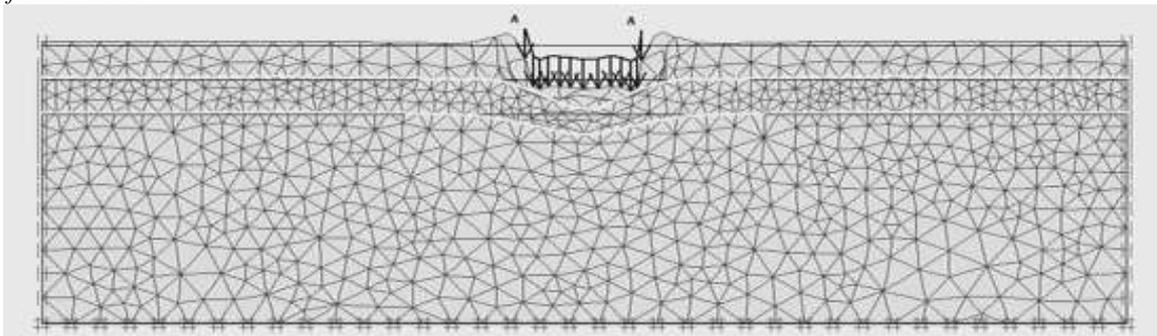
5. One geo-grid is at 2<sup>nd</sup> another one is at 3<sup>rd</sup> layer i.e. at 1.75 in and 0.875 in respectively from the top of the foundation
