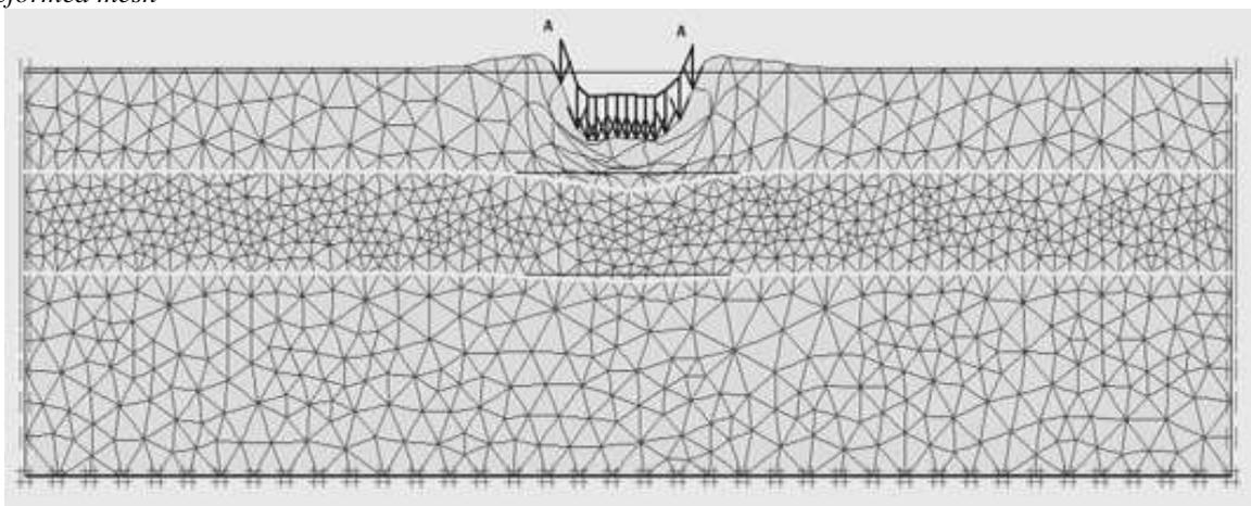
6. Two geo-grid is at 3.5<sup>th</sup> layer of soil i.e. at 0.4375 inch from the top
